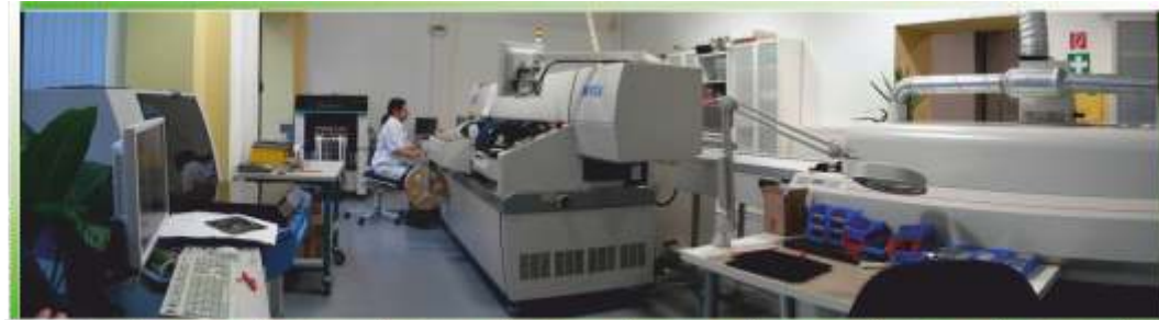
ZIMO production machine room: two placement robots, Reflow soldering oven, soldering-paste printer, AOI device.
