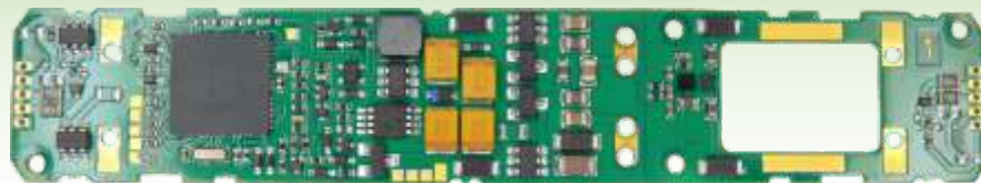
Customized loco decoder for Roco N scale Taurus
