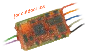
MX820D same as MX820E, but with a water- proof shrinking tube
