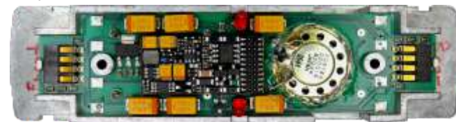
Loco adapter board for a swedish „Class Du“ with sound decoder MX644 (MTC interface) plugged-in. The board includes energy storage containing 6 Tantalum capacitors.
