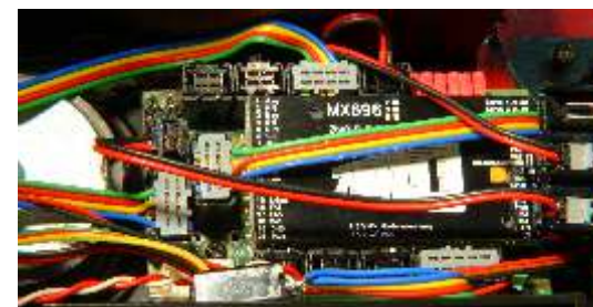
Trainline HSB Mallet, installation of loco board LOKPLSHMAL and inserted Large scale Sound decoder MX696S
