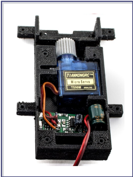
Next generation DCC Many features Situated in the LGB switch drive chassis
